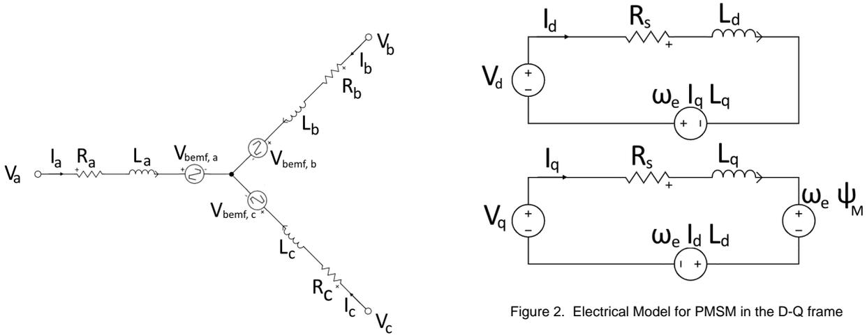
Figure 1. Electrical Model for PMSM
