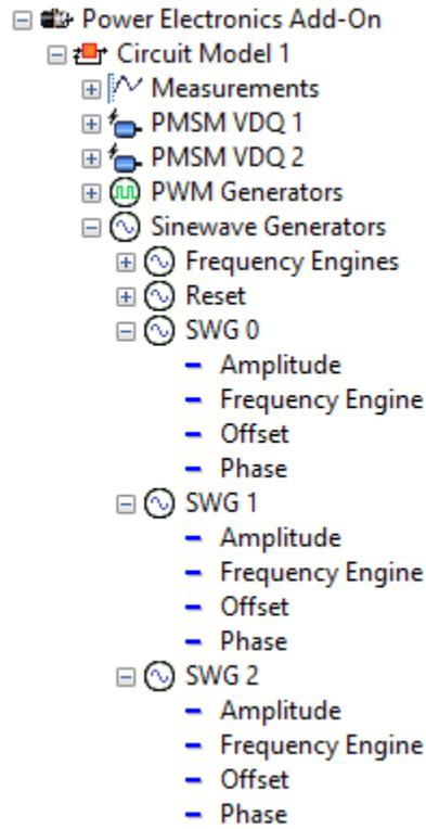
9. **Save** the System Definition file and run the simulation. The voltage source blocks in the circuit model will behave as a synchronized three phase voltage source with a 120 degree phase shift between each signal.
