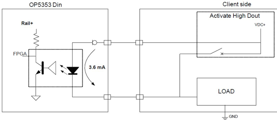
Typical low side open circuit detection
