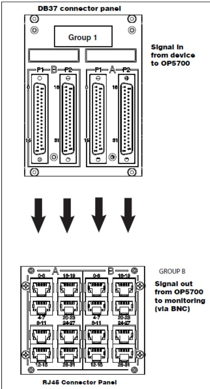
Two DB37F connectors (P1 and P2) are available for each mezzanine, and their pinout depends on the type of mezzanine installed:
