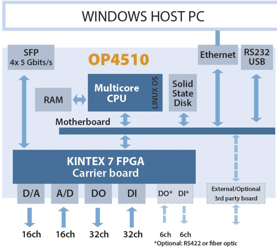
A series of standardized I/O configurations are available with the OP4510 V2, each targeting specific applications. There are also several options for external boards to expand the OP4510 V2 capabilities: CAN communication, synchronization (IRIG-B, PPS or IEEE1588) or I/O expansion. (See OP4510 V2 I/O Expansion Options in [OP4510 V2 Rear Interface](#) for full details).
