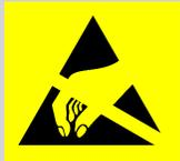
**JTAG connector is highly sensitive to ESD.** Always leave plastic plug in place when not in use. Wear anti-static wrist strap at all times when using this connector.
